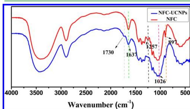
Figure 3. FTIR spectra of the NFC and NFC–UCNPs.
