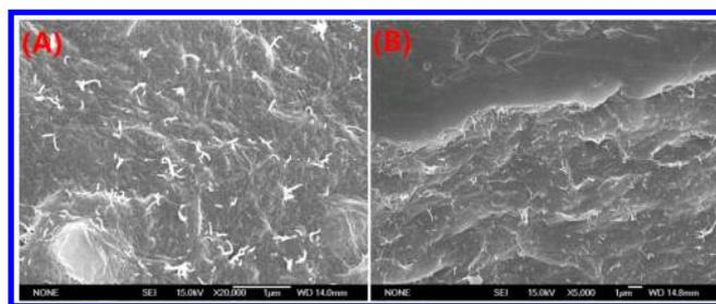
Figure 4. SEM images of the (A) surface and (B) fracture section of NFC–UCNPs nanopaper.
